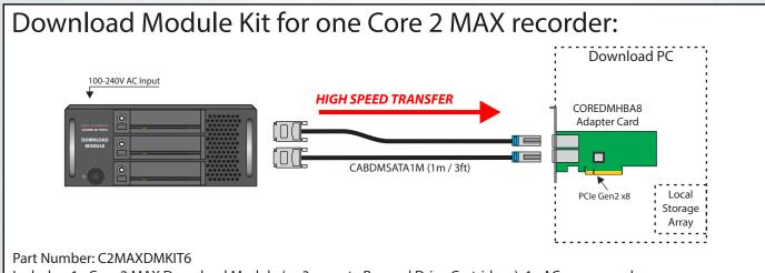
Includes: 1x Core 2 MAX Download Module (w. 3x empty Rugged Drive Cartridges), 1x AC power cord, 2x CABDMSATA1M cables, and 1x COREDMHBA8 adapter card (PCIe Gen2 x8)
